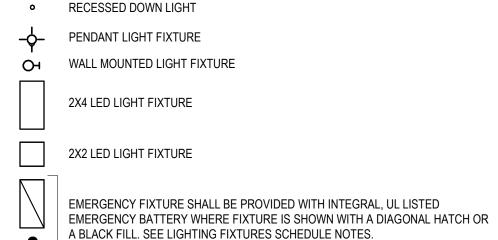
REMOTE FIXTURE POWERED BY ADJACENT EMERGENCY EGRESS FIXTURE
