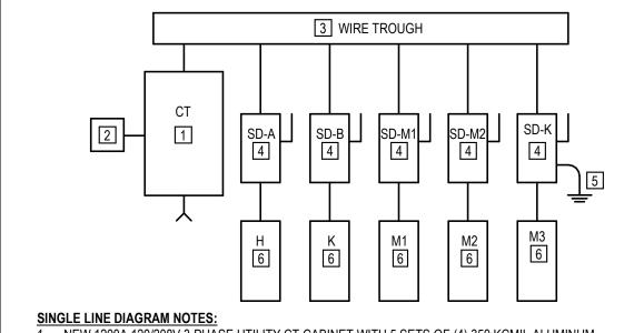
1. NEW 1200A 120/208V 3-PHASE UTILITY CT CABINET WITH 5 SETS OF (4) 350 KCMIL ALUMINUM CONDUCTORS IN (5) 3" CONDUIT (EMT WHEN ABOVE GRADE / PVC WHEN BELOW GRADE) UP TO THE UTILITY SERVICE POINT.
